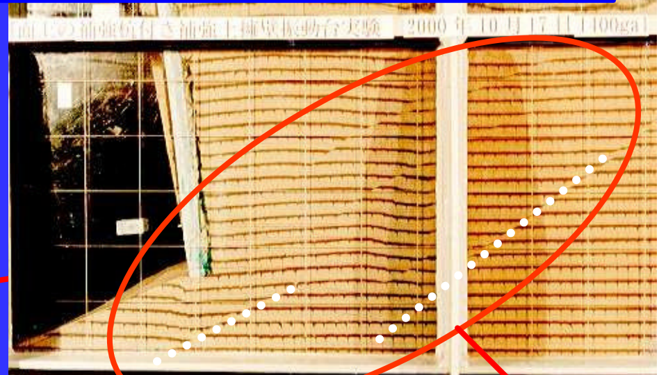
Reinforced with nails( 1.5G)
