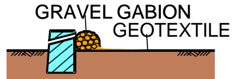
2) PLACING GEOTEXTILE AND GRAVEL GABION
