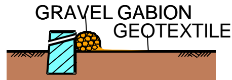
2) PLACING GEOTEXTILE AND GRAVEL GABION
