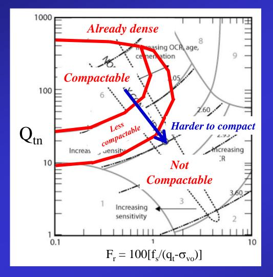
Soils suitable for vibro-compaction essentially plot in SBT zones 5, 6 and 7 on the normalized SBTn chart by Robertson (2009)
