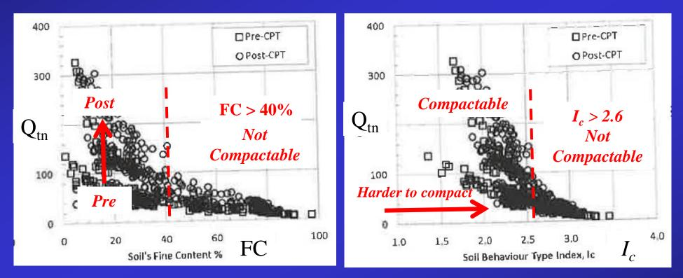
Sandy soils with high fines content (> ~40%) and high CPT  $I_c$  ( $I_c$  > 2.6) are *generally* <u>less compactable</u>
