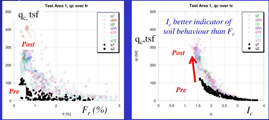
Sandy soils with high fines content and high CPT  $I_c$ ( $I_c > 2.6$ ) are *generally <u>not compactable</u>*
