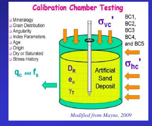
Controlled test environment to study link between CPT  $q_c$  and relative density  $D_r$  in clean sands Since cone resistance varies with overburden stress – it requires 'normalization' to account for depth
