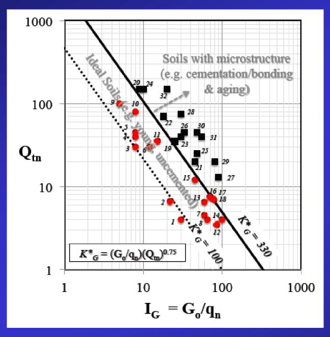
Identify 'unusual' soils - soils with microstrcuture based on SCPT  $G_o = \rho (V_s)^2$
