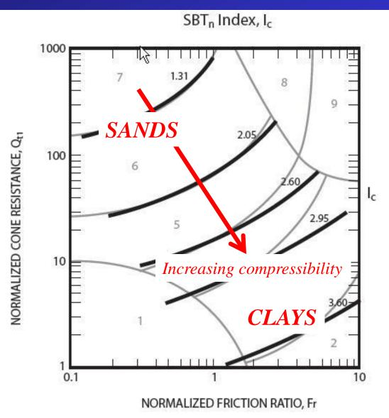
Soil Behavior Type Index,  $I_c$ Ic =  $[(3.47 - \log Q_t)^2 + (\log F + 1.22)^2]^{0.5}$
