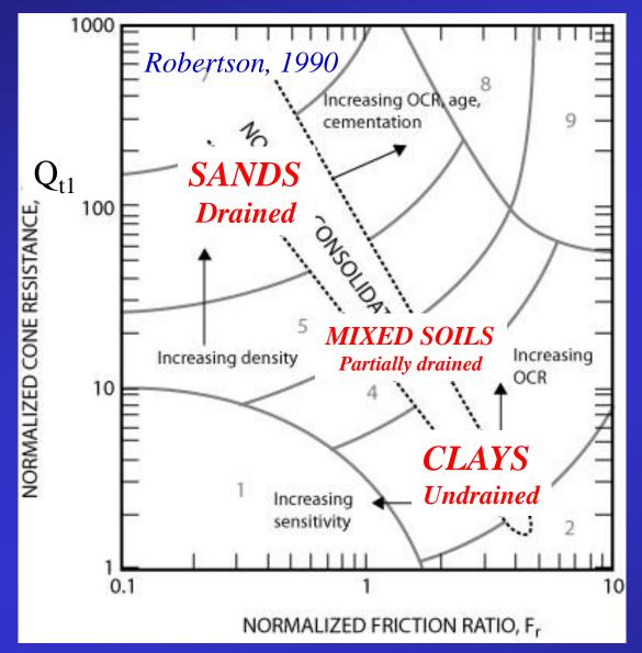
CPT SBT based on in-situ soil behavior (strength, stiffness, *compressibility*) not the same as traditional 'classification' based physical *characteristics* (Atterberg limits, grain size) on disturbed samples
