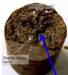
Blocky structure = planes of weakness; evidence of desiccation
