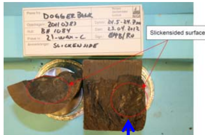
Slickensides are isolated within diameter of sample
