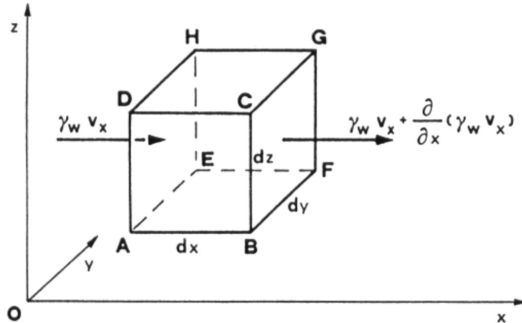
$$F = \left[ \gamma_w v_x + \frac{\partial(\gamma_w v_x)}{\partial x} dx \right] dy \cdot dz - \gamma_w v_x dy \cdot dz = \frac{\partial(\gamma_w v_x)}{\partial x} dx \cdot dy \cdot dz$$
